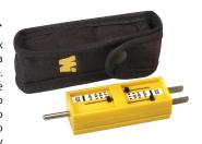
insulated in an impact-resistant plastic housing and is safe to use on energized receptacles. Each blade has an independent spring to relieve stress and assure consistent readings over a long life. When tension falls below 10 oz, monitor the receptacle closely for further deterioration. Tension of 4 oz is the lowest point which a receptacle should be allowed to remain in service. NFPA Standard 99-1996.
